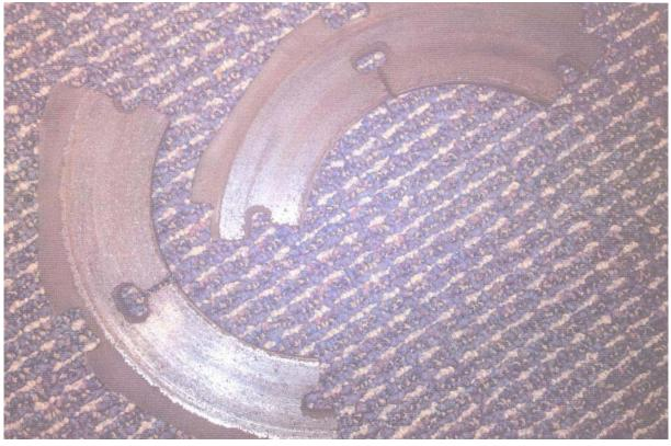
Pilatus PC 1247 Failed Brake Disk, ATA 3242
